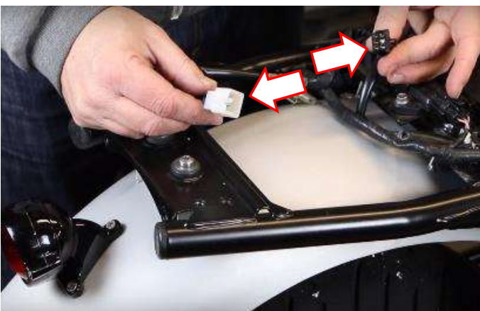
Connecter sur la moto Connect onto the bike's loom
