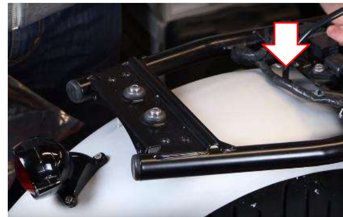
Percer et faire passer le faisceau Drill and pass the loom through
